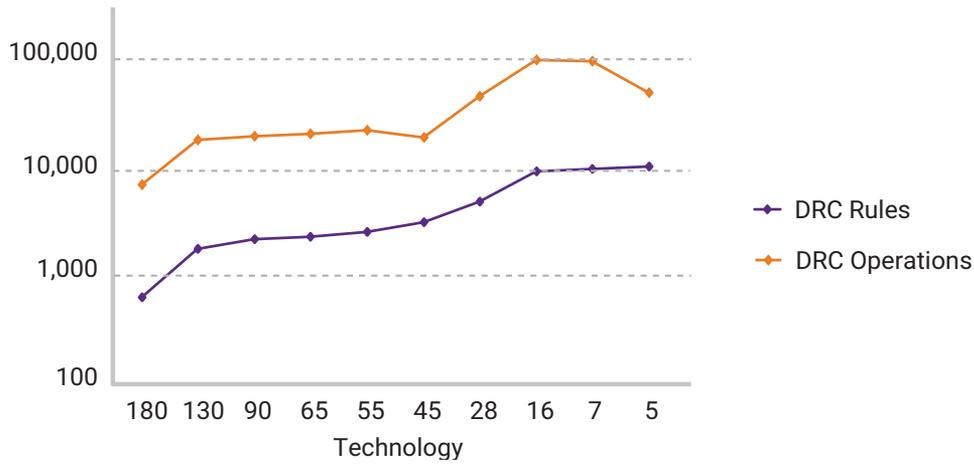
Figure 2: Increasing DRC complexity
